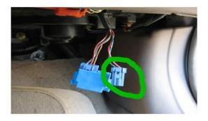
There is no OBD port on the Honda SMX, diagnostics of the Transmission Light is done via flash codes.
