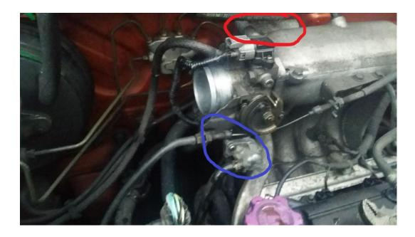
The Rear Idle control valve is held in with 2 bolts on the back of the intake manifold (Red), and there is an electrical connector to unplug. Here is an example of one that's DIRRRTY! Clean this carb cleaner to de-coke/clean. Refit when its dry
