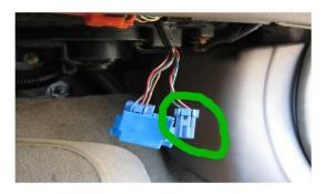
There is no OBD port on the Honda SMX, diagnostics of the Engine Management Light is done via flash codes.
