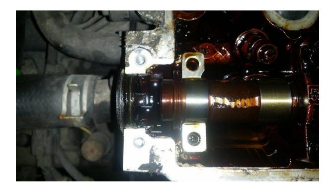
You can then access the end seal cap, remove it and clean away the oil. Clean both the head and cam clamp surfaces where the end cap sits.
